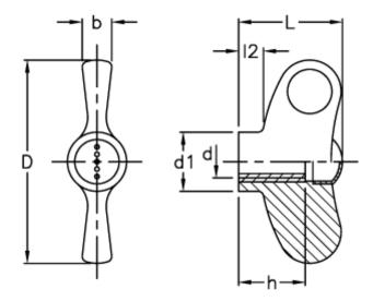
$$\begin{array}{lll} b & = 7 \\ D & = 47 \\ d1 & = 13.5 \\ d \ 6H = M6 \\ h & = 12 \\ L & = 24 \end{array}$$
